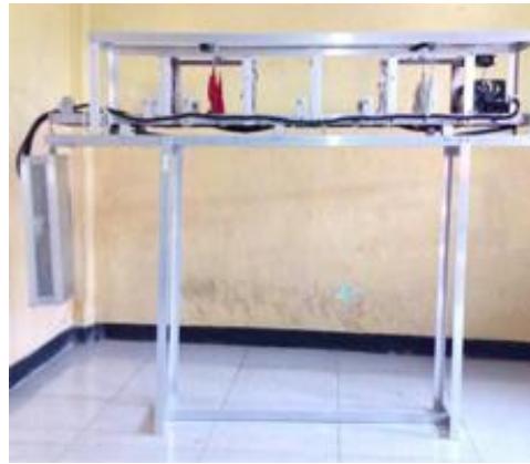
Gambar 9. Prototipe cuci mobil otomatis berbasis sensor LDR
