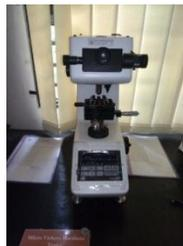
Gambar 4 *Microhardness tester* model FM-300
