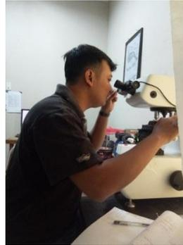
Gambar 3 Proses Uji Kekerasan *Vickers*
