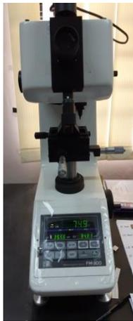
Gambar 1. Alat Uji Kekerasan *Microhardness Tester* Model FM-300
